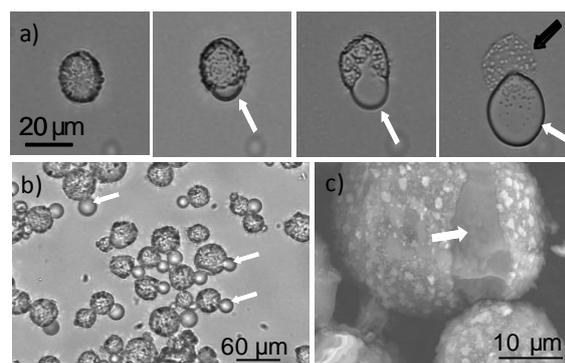
a) Sequence images performed with optical microscopy that depicts the opening of a single shell and the subsequent delivery of the oil when  $T > T_{\text{melting}}$ . b) optical microscopy of several capsules while the oil is out. c) SEM visualization of a capsule in the process of breaking its surrounding shell, induced by the heat of the electron beam. White arrows indicate the liquefied wax, while the black ones indicate the resulting hollow silica shell.
