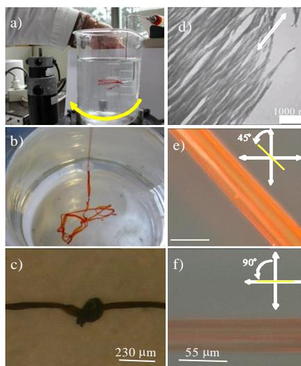
a)  $V_2O_5$  gel under extrusion, b)  $V_2O_5/PVA$  composite fiber under extraction from the rotating beaker, c) fiber forming a knot, d) fiber mesostructure observed through SEM, e) fiber mesostructure observed with SEM, e-f) fiber observed under cross-polarized microscopy.
