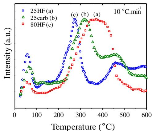
Hydrogen desorption curves obtained through programmed desorption with temperature (primary vacuum heat rate of 10°C min<sup>-1</sup>) and coupled with a mass spectrometer ( $m/z = 2$ ). Li(BH<sub>4</sub>)@80HF (a), Li(BH<sub>4</sub>)@25Carb (b), Li(BH<sub>4</sub>)@25HF (c).
