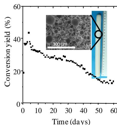
Uni-axial flux catalytic properties of the Col[C-TL-lipase@gGly mo-Si(HIPE)] column for the transesterification of the glyceryl trinoleate with ethanol (40°C in heptane). The curve represents the conversion yield evolution versus time under a debit of 0.1 mL min<sup>-1</sup>.
